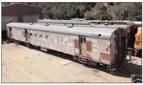
Left: The original UP passenger paint, covered by MOW green. Above: RPO 5901 completely stripped, with the roof painted.
