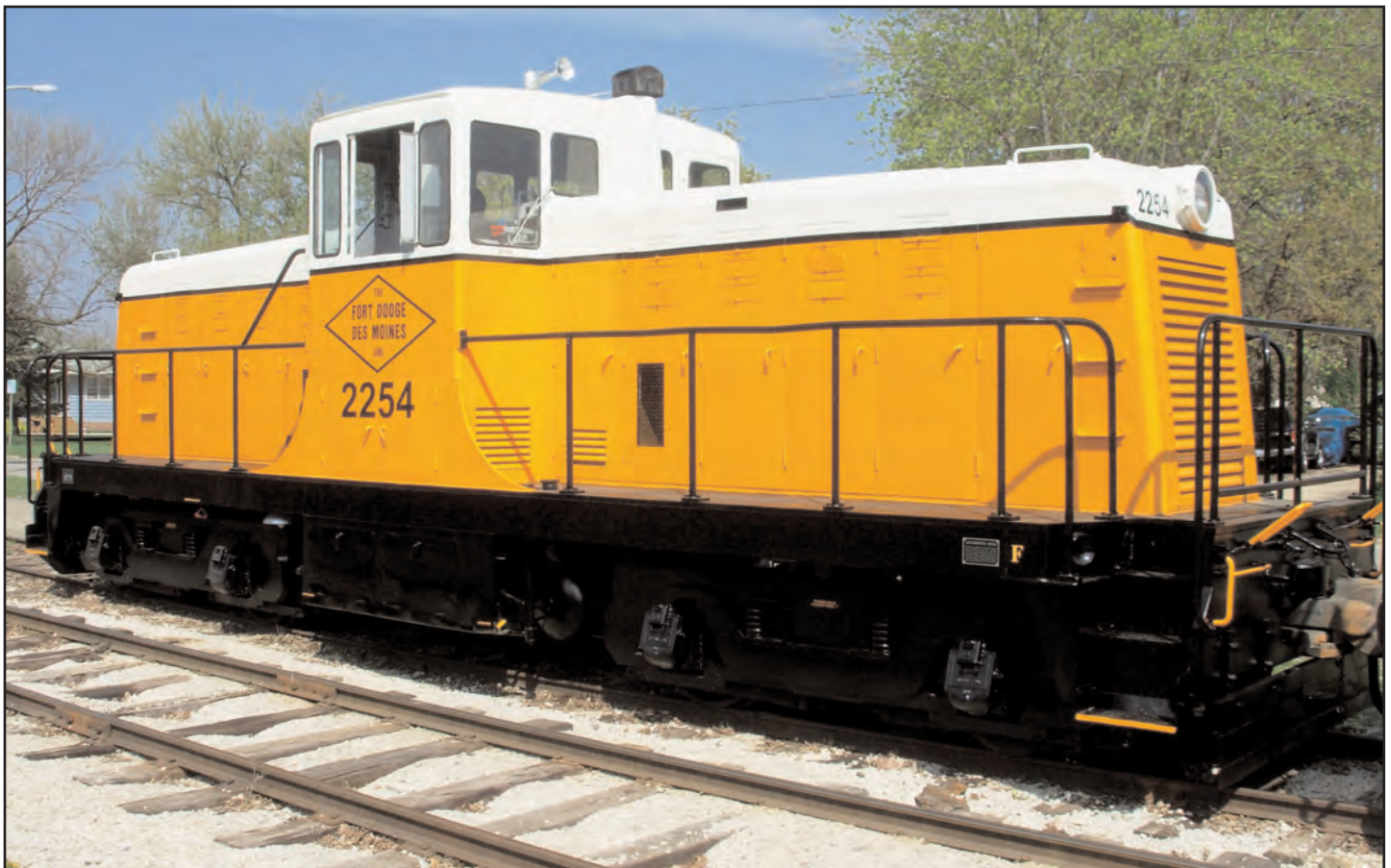
The Boone and Scenic Valley's latest restoration is 80-ton Air Force center cab #2254 (GE 1943). It was the railroad's first locomotive, and is now wearing the diesel color scheme of former interurban Fort Dodge, Des Moines, and Southern, on whose rails the railroad operates. B&SV photo.
