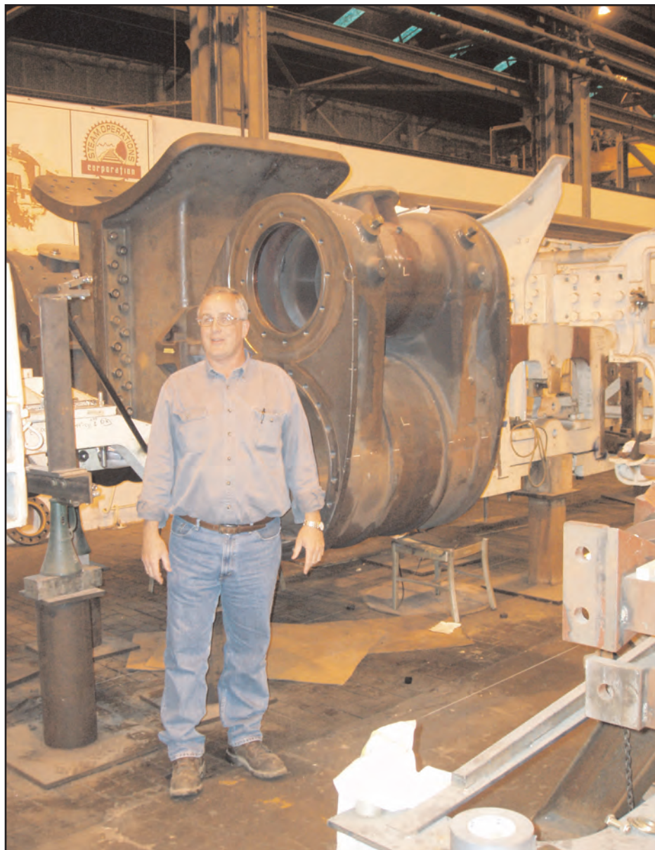
Scott Lindsay with the frame and newly cast cylinders for Austin Steam Train's ex-Southern Pacific 2-8-2 #786.
